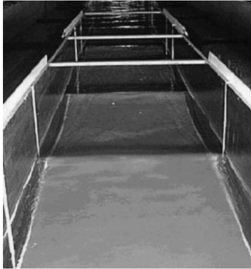
Figure 10. Undular bore experiment. View from the upstream end of the canal.
